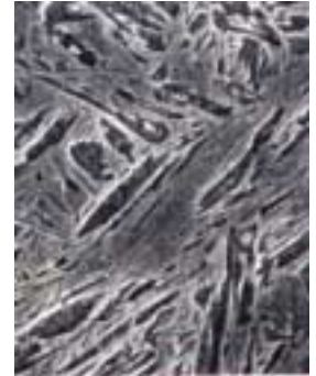
500 HB Water quenched Microstructure
